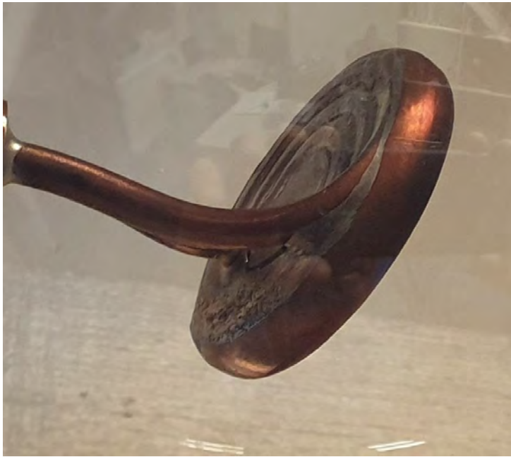
Close up of the water cooled Anode
