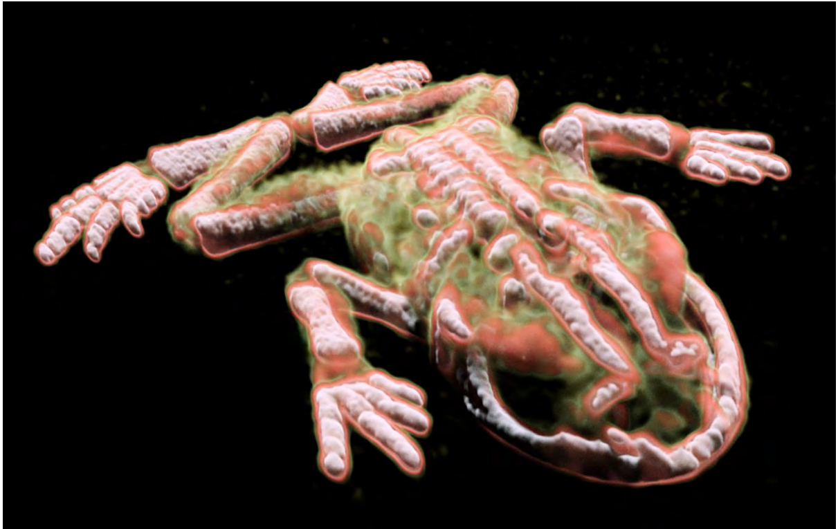
3D image taken on the MARS scanner, pixel size 70 micron x,y,z
